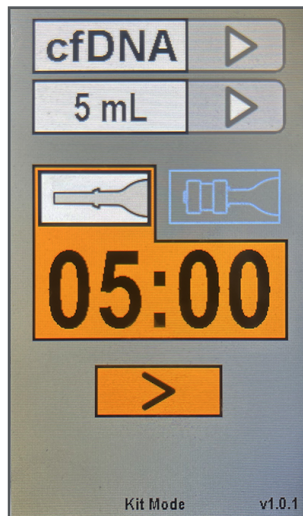
Figure 11 - GUI for cfDNA bead binding on the Revolution Plus
