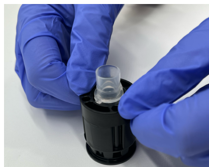
Figure 4 - Releasing the Capture Tube from the Mag Capsule Place the Mag Capsule with the open end of the Capture Tube facing upward on a laboratory benchtop and press down; the Capture Tube will click as it moves upward slightly and is released from the Mag Capsule. The Capture Tube may now be removed from the Mag Capsule by gripping the Capture Tube and pulling it upward gently away from the Mag Capsule.
