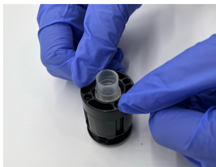
Figure 4 - Releasing the Capture Tube from the Mag Capsule Place the Mag Capsule with the open end of the Capture Tube facing upward on a laboratory benchtop and press down; the Capture Tube will click as it moves upward slightly and is released from the Mag Capsule. The Capture Tube may now be removed from the Mag Capsule by gripping the Capture Tube and pulling it upward gently away from the Mag Capsule.
