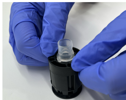
Figure 4 - Releasing the Capture Tube from the Mag Capsule
